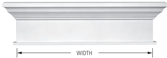
11-311 Window Head 11-311-__-WD Window Head with Dentil Trim* Ht. 14" Proj. 5" Widths available: 44", 68", 76", 78", 80", 104", 115"
